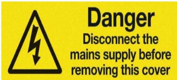
This label is found on the lid of the electric box. Before removing the electric box lid make sure that the cabinet is isolated from the incoming 230v supply. The cabinet isolator is located at the right hand end of the electric box
